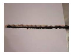
This step can be optional, but to provide better conduction for the probe, a strip of Aluminum foil tape can be cut and rolled up to fill in the groove above the probe.
