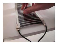
Next, cut off two pieces of the electrical tape and cover the metal connectors with it. This will prevent the risk of electrical shock. Flexwatt heat tape also typically comes with plastic insulators for this same
